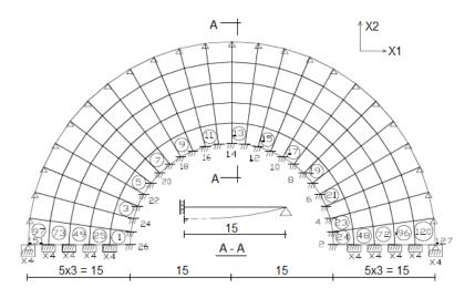
Geometry: Radius: • internal: 15.0 • external: 30.0 Thickness: 0.5 Modulus of Elasticity: 3.0x10<sup>7</sup> Poisson ratio: 0.3
