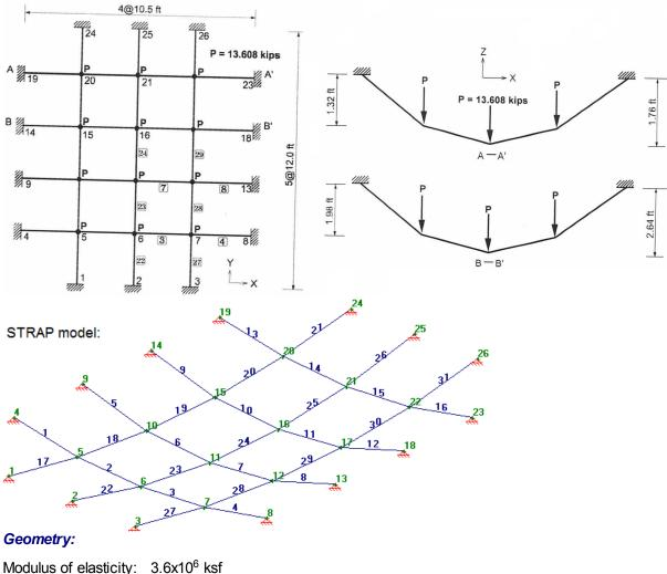
Poisson's ratio : 0.0 Cable area: 0.01 ft<sup>2</sup> Supports: exterior nodes: all DOFs fixed
